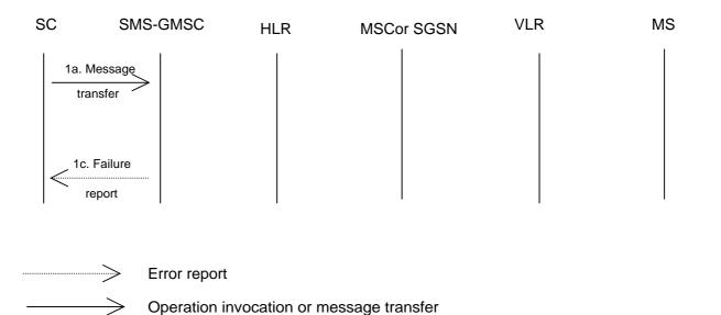
Figure 03.40/15b): Short message transfer attempt failing due to error at the SMS-GMSC
