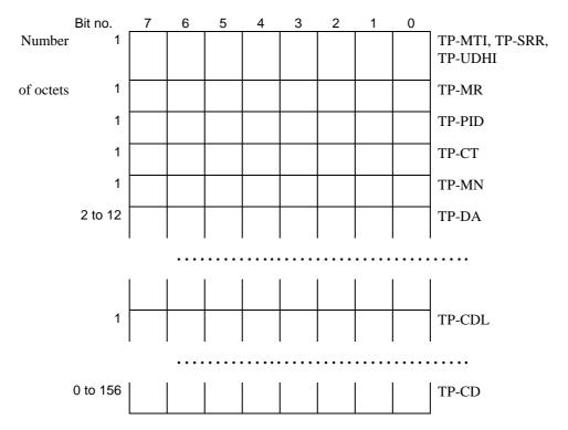
NOTE: The maximum guaranteed length of TP-CD is 146 octets. In order to achieve the maximum stated above (156 octets), the TP-DA field must have a length of 2 octets.
