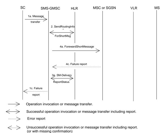
Figure 03.40/15d): Short message transfer attempt failing due to error at the MSC or SGSN
