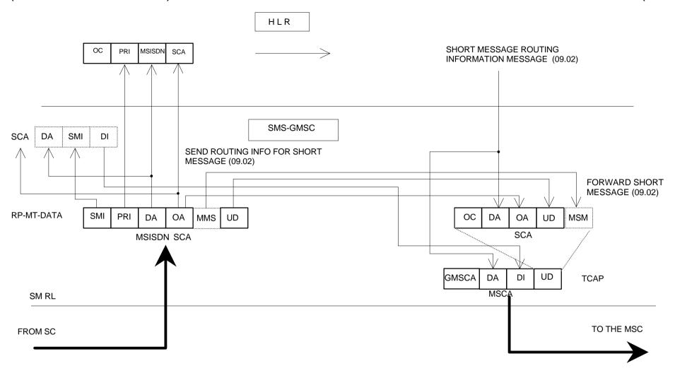
NOTE: A sequence of short messages will have MMS set to 1 in each RP-MT-DATA except the last (last will have MMS set to 0). Each RP-MT-DATA will be carried via FORWARD SHORT MESSAGE via TCAP and will be assigned the same Dialogue Identifier as previous RP-MT-DATAS in the sequence.
