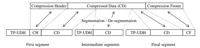
Figure 9.2.3.24.1.(a) Concatenation of a Compressed short message
