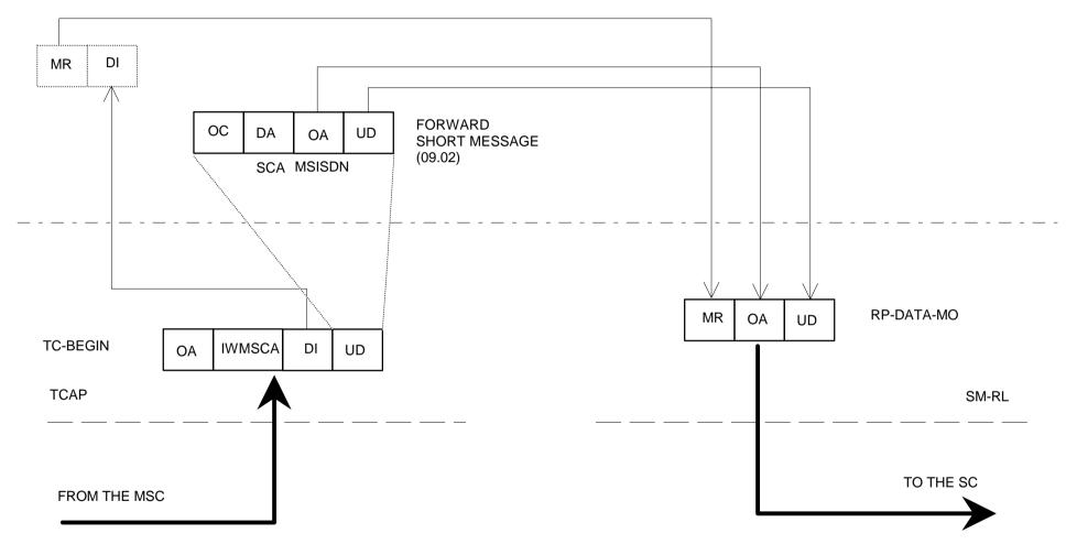
NOTE: MR is of local significance to the IWMSC/SC interface and is not the value supplied by the MS via the MS/MSC interface
