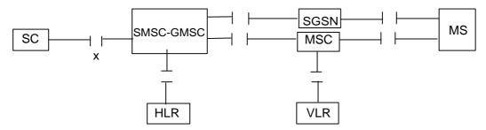
NOTE: Since the short message mobile terminated procedure covers the functionality required at SM-RL for transferring TPDUs from SC to MS, the procedure described covers both short message (SMS-DELIVER) and status report (SMS-STATUS-REPORT) transfer. The term "short message transfer" therefore, in this clause, covers both cases.
