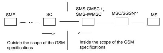
\*): SMS-GMSC when the short message is transferred from the SC to the MS, SMS-IWMSC when the short message is transferred from the MS to the SC. The SC may be integrated with the SMS-GMSC/SMS-IWMSC.
